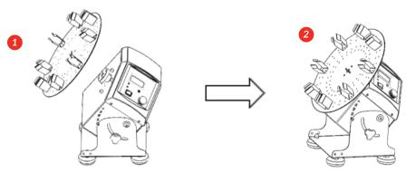
Secure the tube holder disk accessory with the four screws, lock washers and washers (installed in that order) using the included Allen wrench.
